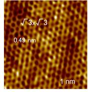
**Figure:** STM image of plumbene on a Pd-Pb alloy thin film on Pd(111)
