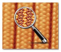
STM image of the 1D DNRs of silicon grown on a silver (110) substrate. The structure reveals that Si arrange as perfect alternating pentagons residing in the missing row troughs of the reconstructed surface Ag (110).
