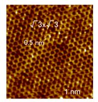
Figure: STM image of stanene on a  $Ag_2Sn$  surface alloy on Ag(111)
