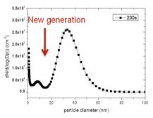
**Figure:** Multi-mode particle size distribution obtained in DC discharge
