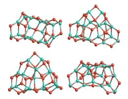
Figure: Low-lying isomers of (Al<sub>2</sub>O<sub>3</sub>)<sub>8</sub>
